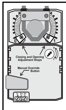
Open and Closed Adjustment Stops
