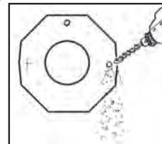
Fig. 30 - Pre-drill for anchors
