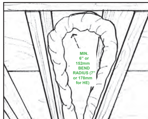
Fig. 17 - 6" (152mm) minimum radius on bends
